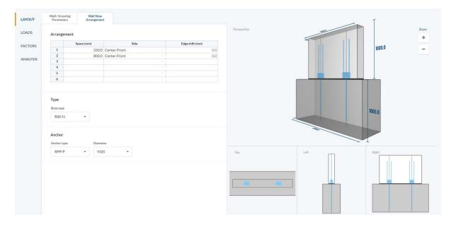
Moving on to the "LOADS" page, the following load values have been selected: an axial load of 20.00 kN, a moment value in the x-direction of 15.00 kN, a moment value in the y-direction of 15.00 kN, a shear value in the x-direction of 10.00 kN, and a shear value in the y-direction of 10.00 kN.
