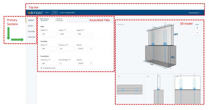
Main structure of the primary sections and associated tabs are given below:
