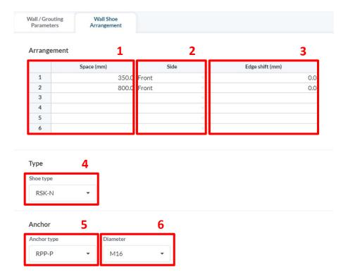
**1** The number of wall shoes and the distance between them can be adjusted by users. The distance for the first shoe is measured from the left edge of the precast wall, and for subsequent shoes, it is measured from the previous shoe. A more comprehensive explanation of the wall shoe arrangement will be provided in the example calculations later on.
