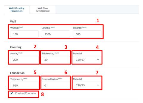
**1** The wall dimensions can be customised by users as needed. Any adjustments made will be automatically reflected in the 3D model on the right-hand side. Below, you will find an explanation of these dimensions.
