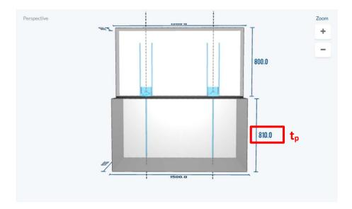
**6** This dimension is associated with the foundation and is measured from the edge of the precast wall on both the right and left sides. Here is an example where a 300mm from the wall edges is required.
