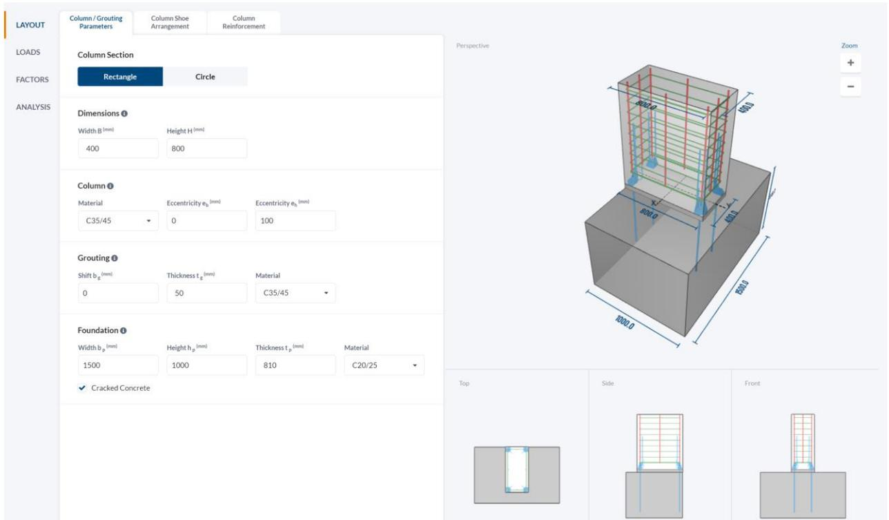
As an example, 400x800 column is defined on the 1500x1000x810 foundation. Column and grouting material selected as C35/45. Column has eccentricity 100 mm on the Y axis. Grouting thickness is 50 mm. Foundation material selected as C20/25.
