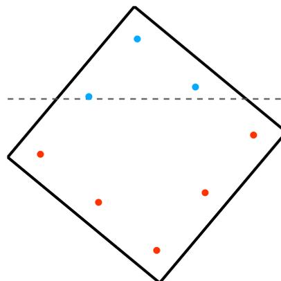
– NA, ● Tensioned bar, ● Compressed bar
