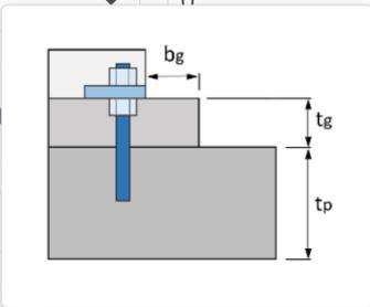
The diagram shows a column cross-section with a grouting layer. The grouting layer has a thickness  $t_g$  and a shift  $b_g$  from the center. The column has a thickness  $t_p$ .
