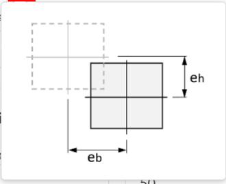
The diagram shows a square column cross-section with a central reinforcement cage. A dashed line indicates the original center, and a solid line indicates the shifted center. The vertical distance between the original and shifted centers is labeled  $e_h$ . The horizontal distance from the original center to the edge of the column is labeled  $e_b$ .
