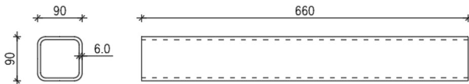
Picture 2. RLK12 slab support dimensions and structure
